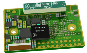
Picture 3: CB-OEMSPA312i-07 OEM Serial Port Adapter short range with internal antenna and Flexfilm connector
